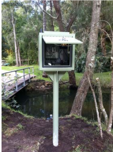
Figure 6: Water Level Gauge (submersible pressure transducer) at Great Mackerel Beach
