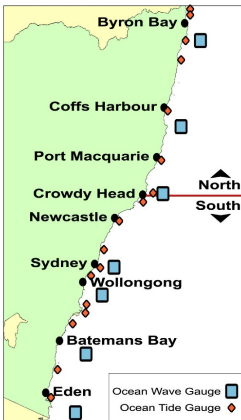
Figure 1: Location of Ocean Wave Buoys and Ocean Tide Gauges relative to Crowdy Head
