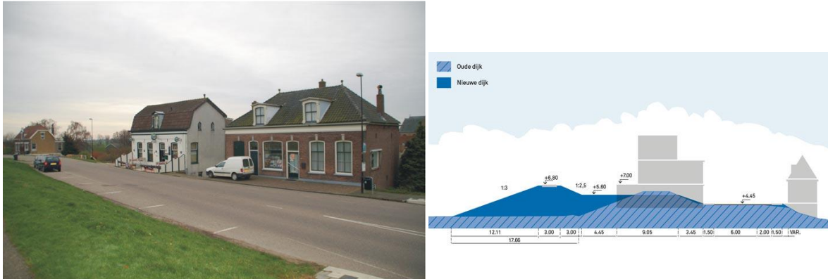
Figure 9 Impression of the location of the multi purpose levee (left) & schematic representation of the levee (right)
