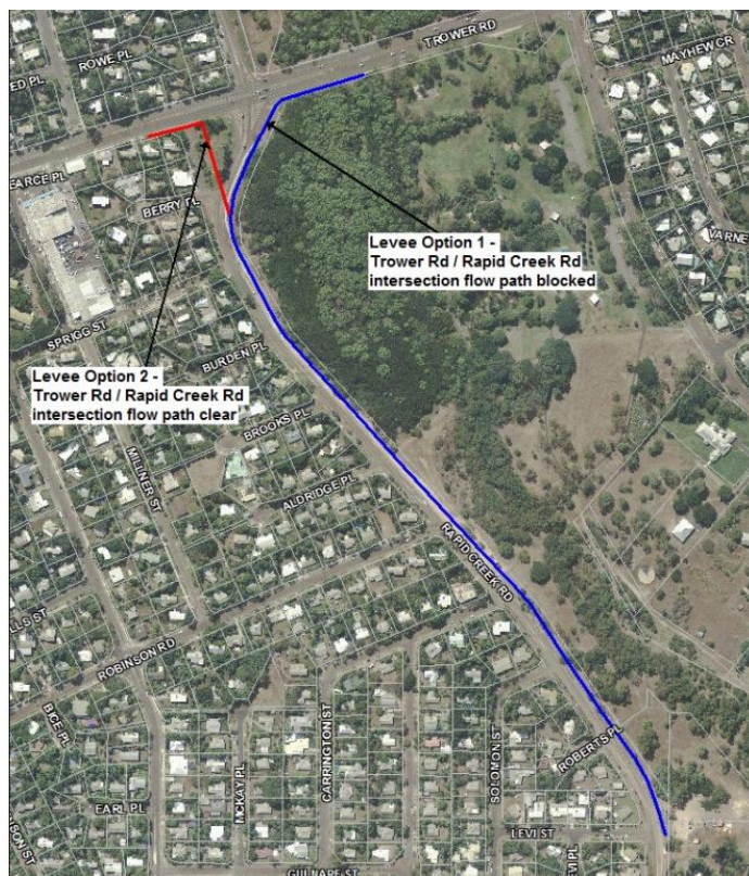
Figure 4 Levee alignment options
