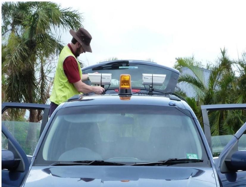
Figure 2: The Rapid Inventory Collection System ( RICS ) mounted on a car
