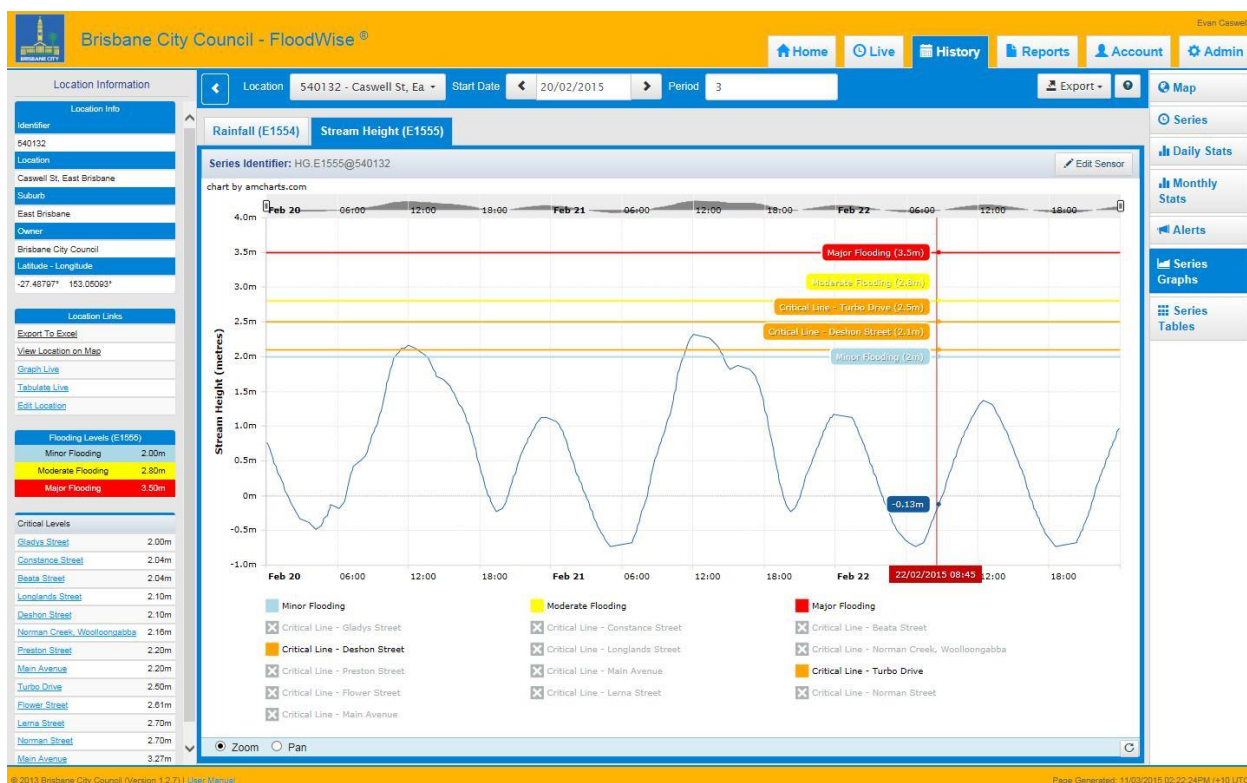
Fig. 2: Typical stream gauge plot with coloured alert trigger levels
