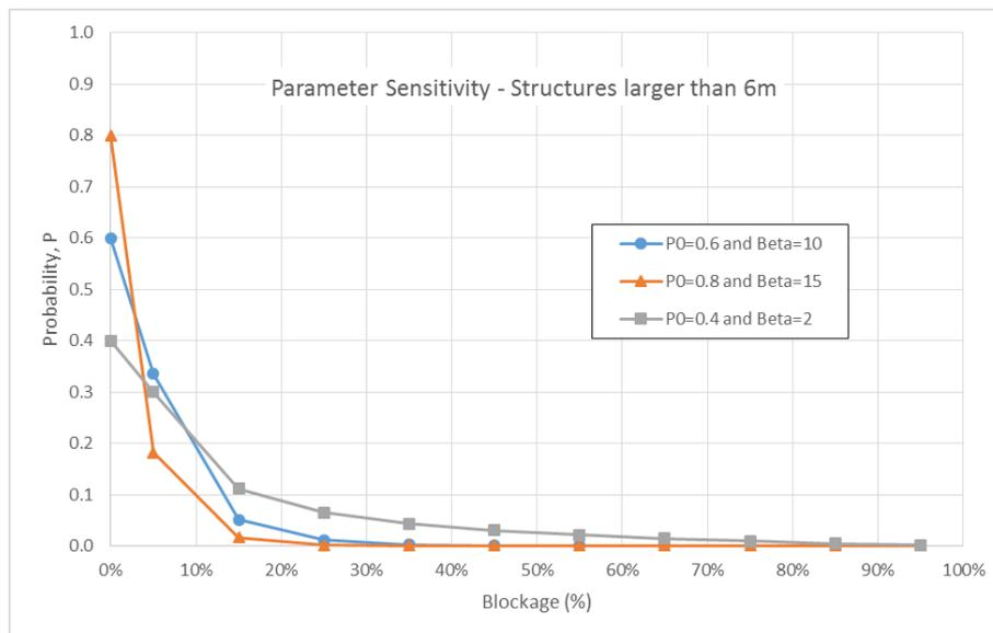
The main result of sensitivity test is the variation in the mean of the distributions. As noted from the results of the stochastic modelling, in most cases the probability-neutral blockage tracked closely with the mean blockage for many sites. These results are summarised in Table 2.
